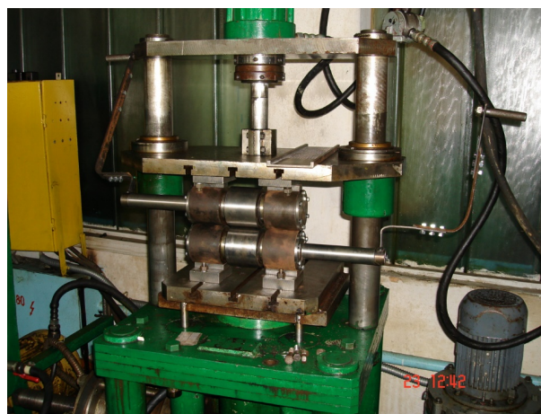
16 the experimental facility sample with hydroimpulsive drive component for vibro-blowing dehydration of food production wastes is created
