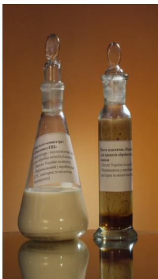
Experimental samples of the working emulsion "Rapломol-EP" and paste-concentrate "Rapломol-P1v" for mechanical processing of metals
