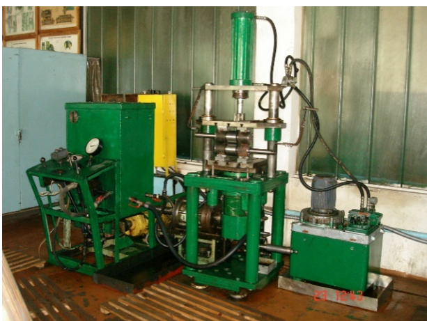
16 the experimental facility sample with hydroimpulsive drive component for vibro-blowing dehydration of food production wastes is created
