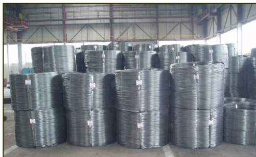
The bundles of reinforcing bars with the strength index 600 MPa
