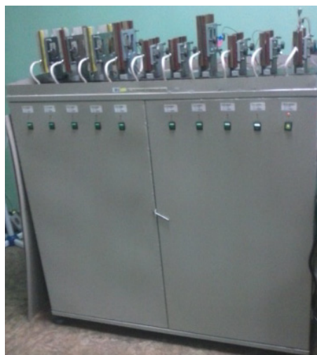
10-channels test device for measuring the parameters of supercapacitor
