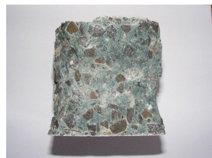
Destruction of the filler after the concrete test
