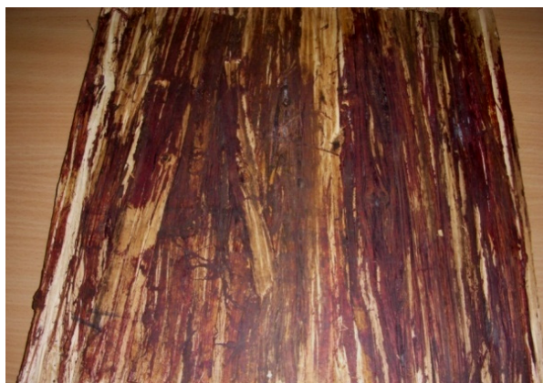
Three-layer wood-composite material on the basis of pressed branches of poplar with perpendicular direction of fibers
