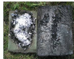
Testing of experimental samples covered with protective coating, under the influence of magnesium flame.
