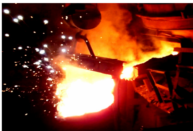
Process of extra-furnace cast iron desulfurization by magnesium reduced from oxide in the volume of liquid melt by virtue of parallel chemical conversions heat
