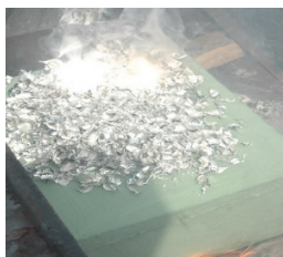
Testing of experimental samples covered with protective coating, under the influence of magnesium flame.
