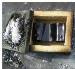
Testing of experimental samples covered with protective coating, under the influence of magnesium flame.
