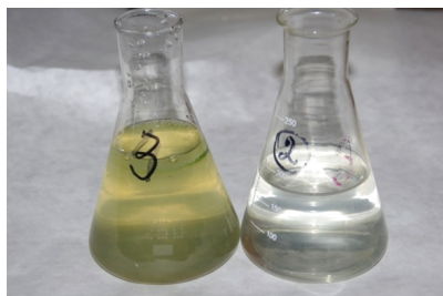
Source swamp water (left) and water purified with the plant (right)
