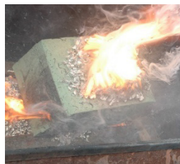
Testing of experimental samples covered with protective coating, under the influence of magnesium flame.
