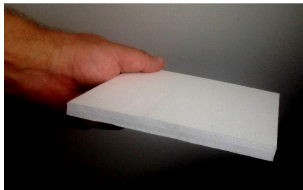
The appearance of the prototype of 11 mm thick non-combustible heat-protective coating
